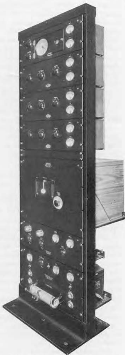
The standard-frequency assembly used in the Michelson experiment was similar to the one shown above, except that one of the multi-vibrators was replaced by an amplifier for the 0.1-second pulses from the synchro-clock
